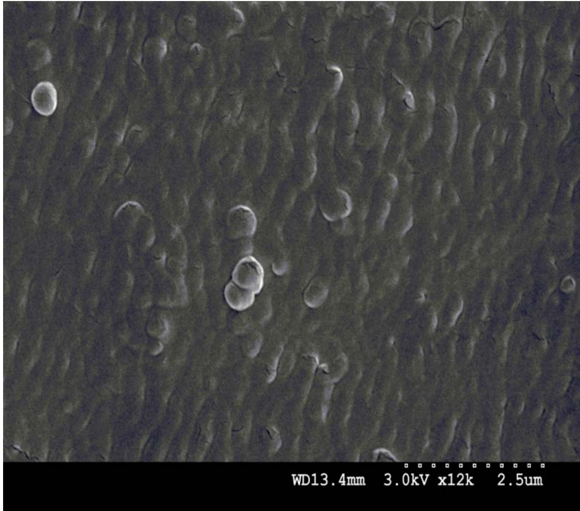
Figure 4.8. Continuous PEGMA coating formed by s-ATRP on surface PP HFM, cleaned by 36 hour extraction with acetone solvent prior to s-ATRP.
